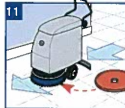
11 When autoscrubbing, overlap the passes and flip or change pad when needed.
