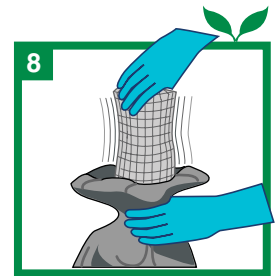
8 Empty or replace vacuum bag into a plastic liner, and check filters every two hours or more as needed.
