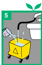
5 Mix the stripper solution properly with cool water.
