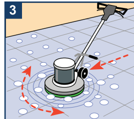
3 Strip or top scrub the floor appropriately before applying any finish. Make sure there is no residue left on the floor. Rinse if needed.
